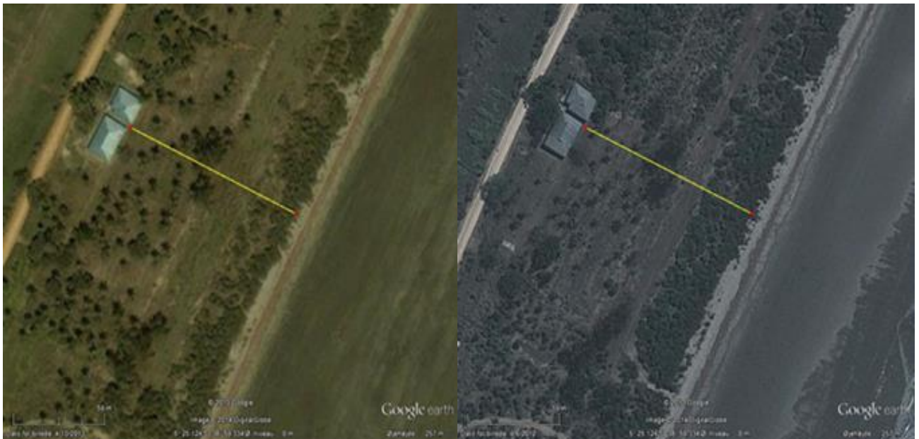
Figure 36: Details of the shoreline north of Pangani River, location indicated by the red dot in Figure 1 14. Left: Oct. 30, 2008. Right: June 9, 2012. The length of the line from the buildings to the shoreline is 120 m.
